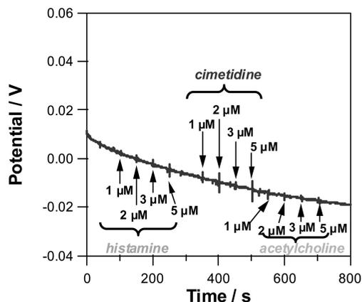
**Figure 4.** Potential versus time plot using an  $\text{IrO}_2$  pH sensor in DMEM buffer while adding histamine, cimetidine, and acetylcholine to achieve solution concentrations 1, 2, 3, and 5  $\mu\text{M}$  each.
