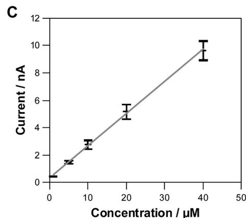
**Figure 2.** Assessment of the BDD electrode for detection of histamine. (A) shows a differential pulse voltammogram of histamine in DMEM buffer. (B) shows a FIA trace obtained with various concentrations of histamine, where three repeated measurements were obtained and the calibration curve obtained from these data are shown in (C). All measurements were conducted using a 40  $\mu\text{M}$  boron-doped diamond microelectrode.
