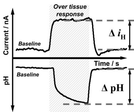
**Figure 1.** Schematic showing example of the traces and data analyzed. The current and pH traces are shown, where the gray-shaded box indicated the region where measurements over the tissue are carried out and the measured parameters,  $\Delta i_H$  and  $\Delta pH$ , are indicated.
